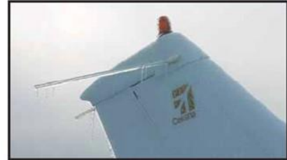
Ice can cause antennas to vibrate so severely that they break
